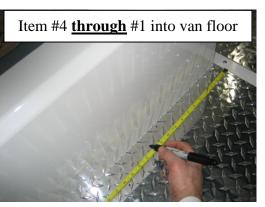
Attach remainder of **Diamond plate floor.** Pre-drill diamond floor (only) w/ 3/16" hole and 1/8" hole through floor of vehicle
